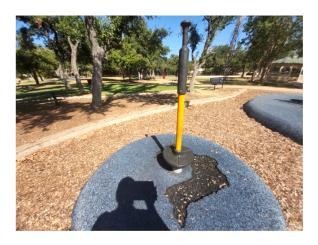
Compliant 2.7.3. Footrests stay in place and pass the protrusion test. (CPSC 12.5, ASTM 8.11.3)
